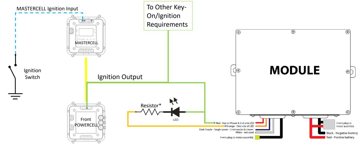
\* Size the value of this resistor based on the maximum current spec for your LED.
