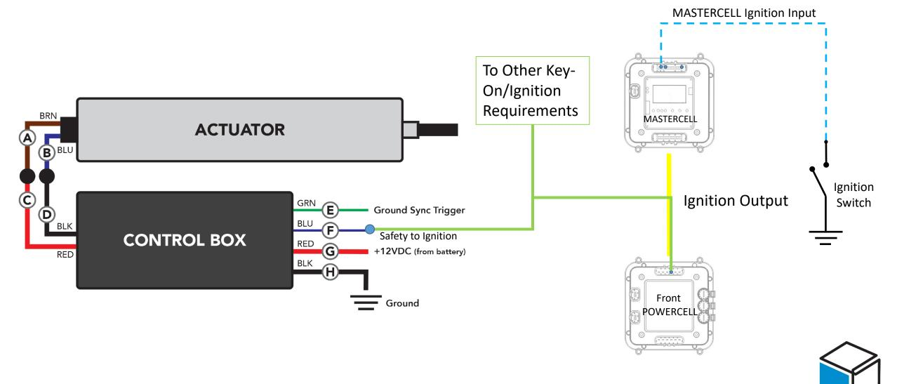
NOTE: Infinitybox Wire Colors & Connector Positions will vary for different kits. See the Configuration Sheet that came with your kit for exact wire colors and locations. Some wires omitted for clarity. Follow the instructions that came with your kit for complete details.
