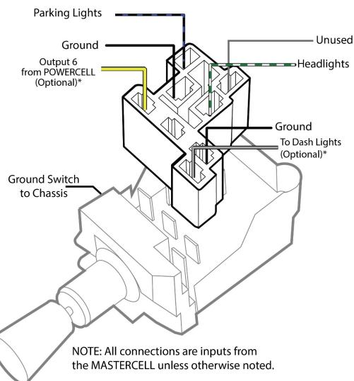
\*This configuration utilizes the built in rheostat in the switch, allowing the dash lights to be dimmed. The dash lights will be on when the parking light output is on.
