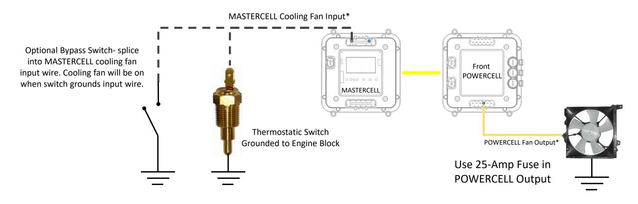
\*NOTE: Infinitybox wire Colors & Connector Positions will vary for different kits. See the Configuration Sheet that came with your kit for exact wire colors and locations.
