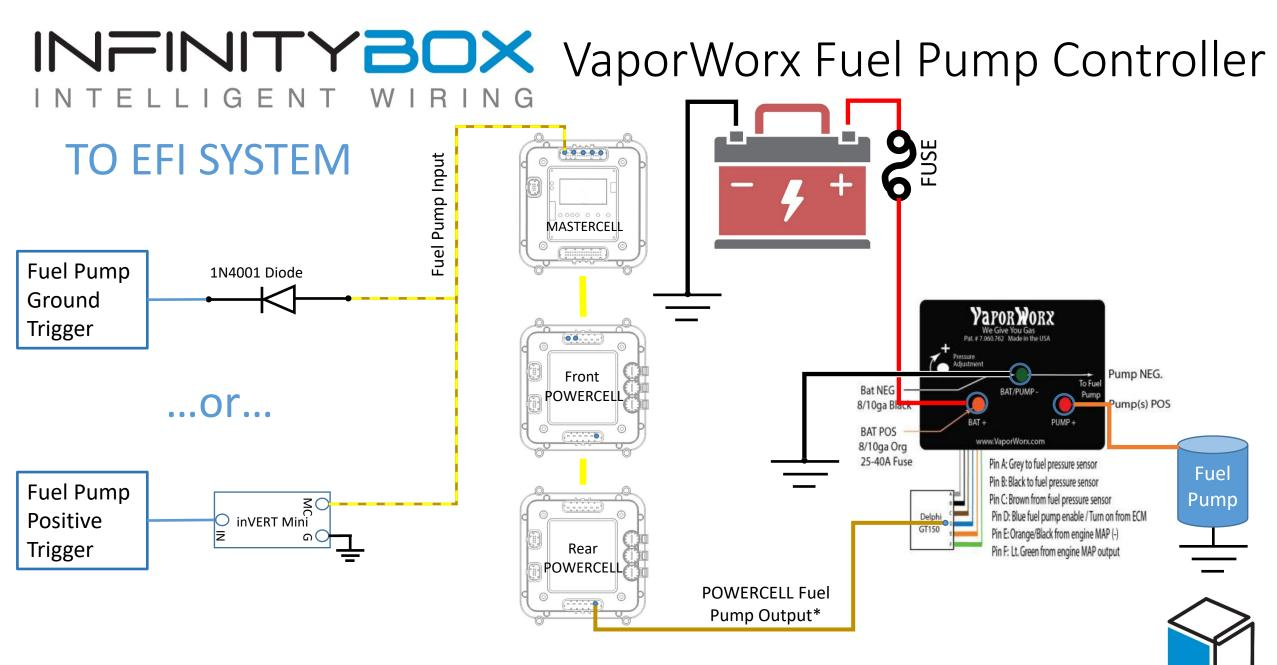
\*NOTE: Infinitybox wire Colors & Connector Positions will vary for different kits. See the Configuration Sheet that came with your kit for exact wire colors and locations. \*\*NOTE: Read and understand the manual that came with your VaporWorx system before wiring. Some wiring omitted for clarity.
