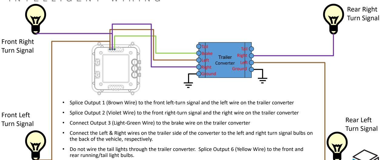
\*NOTE: Infinitybox wire Colors & Connector Positions will vary for different kits. See the Configuration Sheet that came with your kit for exact wire colors and locations. \*\*NOTE: MASTERCELL inputs must be ground switched. Applying 12-volts directly to an input will damage the MASTERCELL and void the warranty.
