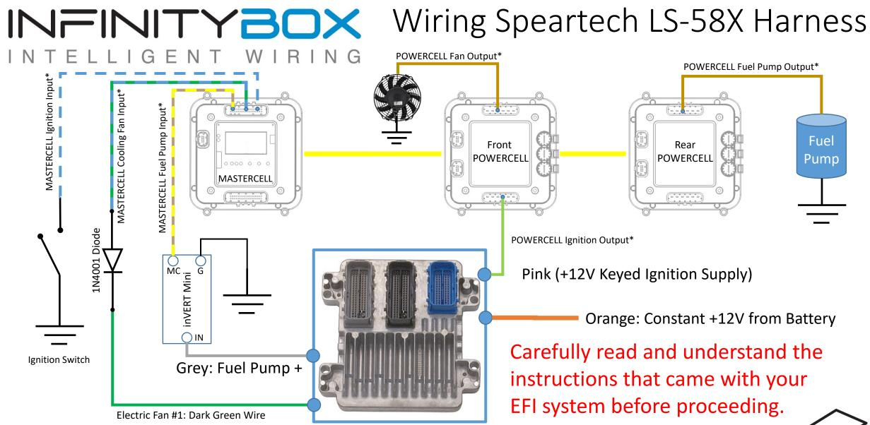
\*NOTE: Infinitybox wire Colors & Connector Positions will vary for different kits. See the Configuration Sheet that came with your kit for exact wire colors and locations. \*\*NOTE: MASTERCELL inputs must be ground switched. Applying 12-volts directly to an input will damage the MASTERCELL and void the warranty. Use an inVERT Mini (as shown) or a relay to convert the fuel pump trigger to a ground trigger for the MASTERCELL.
