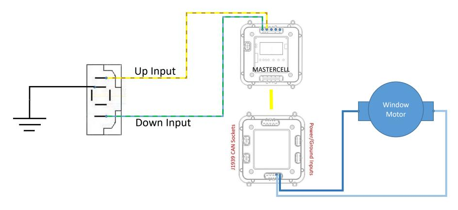
Diagram is shown for the Electric-Life 4980-10-269 Window Switch
