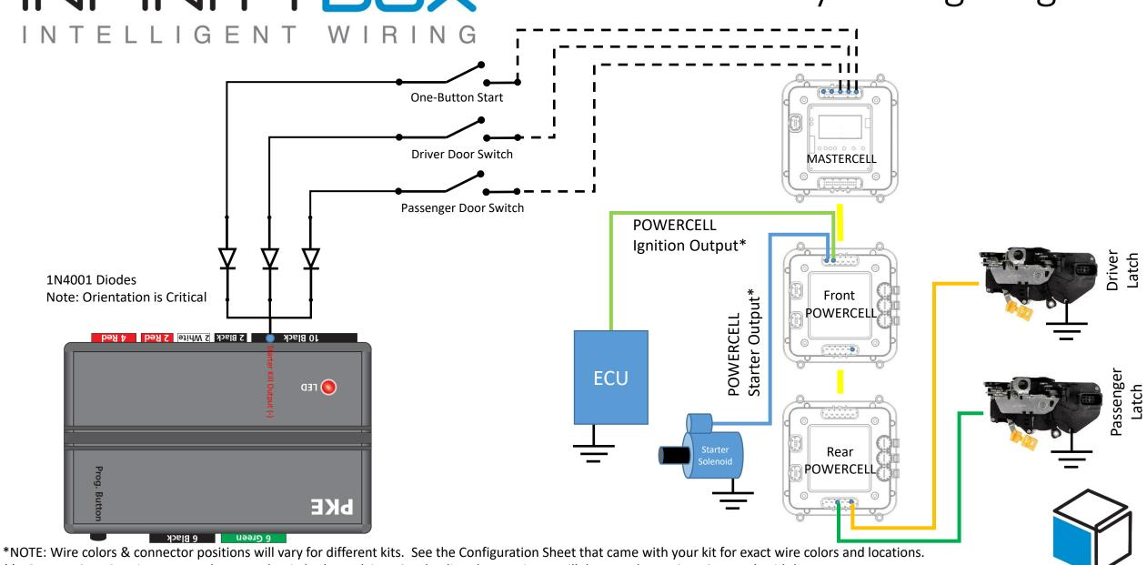
\*\*NOTE: MASTERCELL inputs must be ground switched. Applying 12-volts directly to an input will damage the MASTERCELL and void the warranty.
