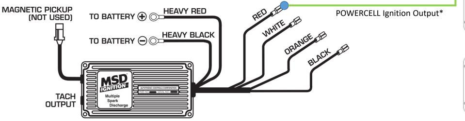
\*NOTE: Infinitybox wire Colors & Connector Positions will vary for different kits. See the Configuration Sheet that came with your kit for exact wire colors and locations.
