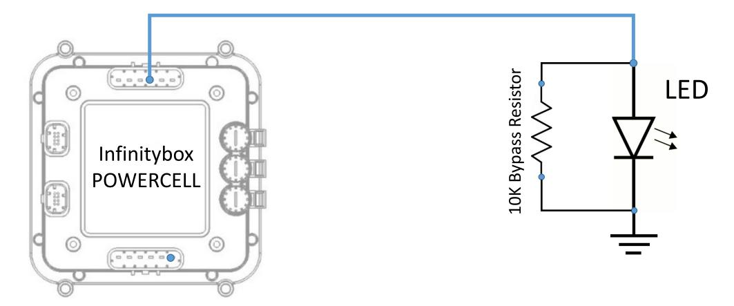
Install 10K (10,000 Ohm) resistor in parallel with your LED to extinguish any dim glowing of the light caused by the POWERCELL diagnostic current.
