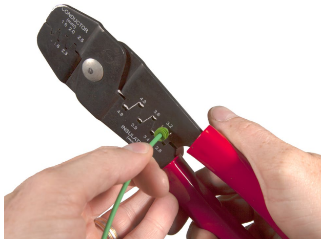
Figure 5. Using a crimp tool to properly connect the terminal to the wire.
