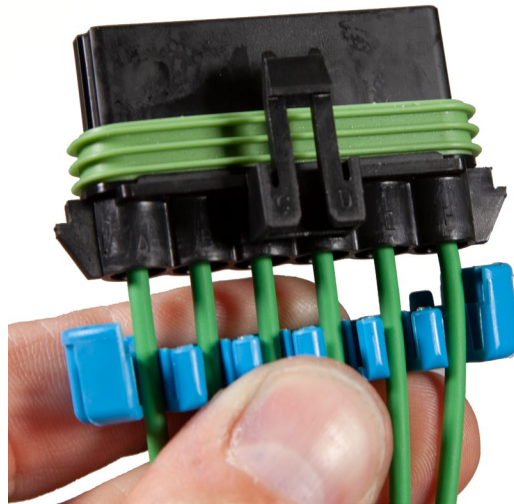
Figure 9. Installing the TPA on the Splice Saver Connector.
