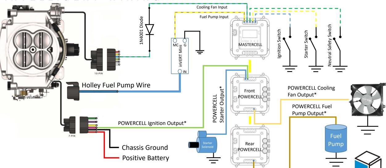
\*NOTE: Infinitybox wire Colors & Connector Positions will vary for different kits. See the Configuration Sheet that came with your kit for exact wire colors and locations. \*\*NOTE: Read and understand the manual that came with your EFI system before wiring. Some wiring omitted for clarity.
