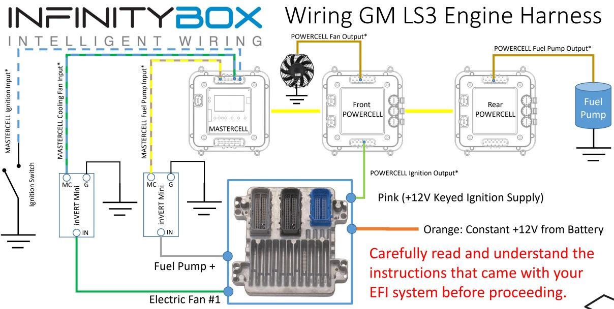
\*NOTE: Infinitybox wire Colors & Connector Positions will vary for different kits. See the Configuration Sheet that came with your kit for exact wire colors and locations. \*\*NOTE: MASTERCELL inputs must be ground switched. Applying 12-volts directly to an input will damage the MASTERCELL and void the warranty. Use an Infinitywire inVERT Mini (as shown) or a relay to convert the fuel pump trigger to a ground trigger for the MASTERCELL.
