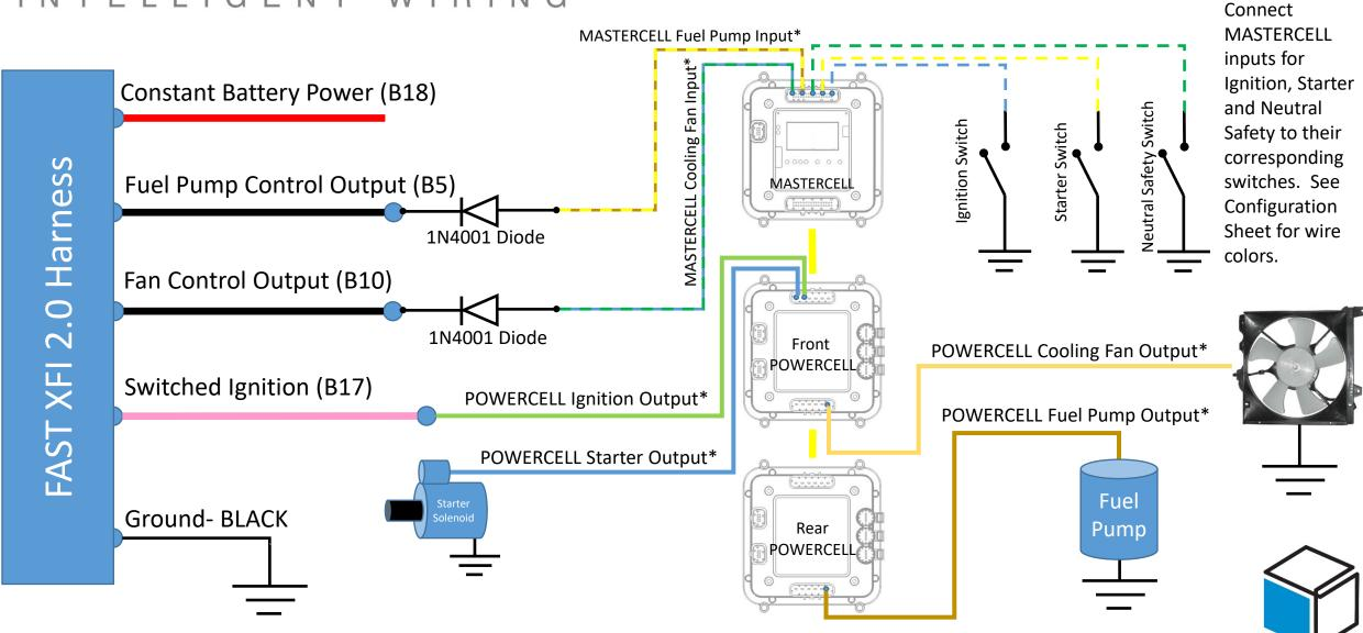
\*NOTE: Infinitybox wire Colors & Connector Positions will vary for different kits. See the Configuration Sheet that came with your kit for exact wire colors and locations.
