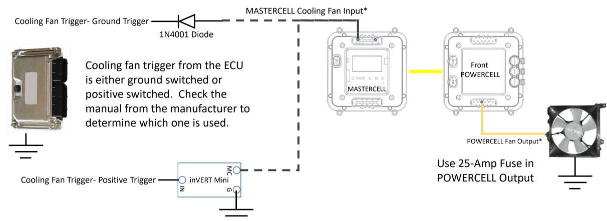
\*NOTE: Infinitybox wire Colors & Connector Positions will vary for different kits. See the Configuration Sheet that came with your kit for exact wire colors and locations. \*\*NOTE: MASTERCELL inputs must be ground switched. Applying 12-volts directly to an input will damage the MASTERCELL and void the warranty. Use an Infinitywire inVERT Mini (as shown) or a relay to convert the fuel pump trigger to a ground trigger for the MASTERCELL.
